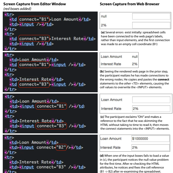
Figure 6: Most errors encountered could be identified and diagnosed by simply reloading the web page. This participant had the longest sequences of such activity. Other errors were harder to detect, requiring the user to experiment with different data values or manually inspect code to diagnose.
