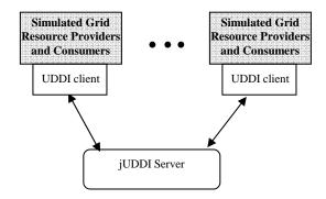
Figure 4. Architecture used for UDDI Evaluation
